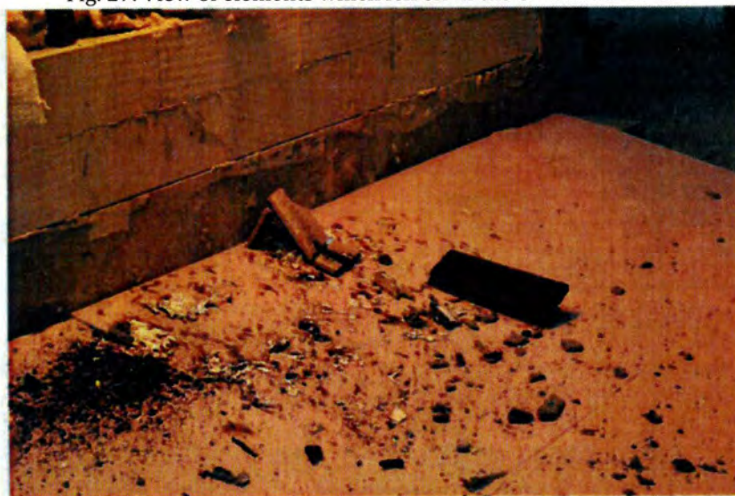
Fig. 28. View of elements which had fallen off before the 10 th minute of test
